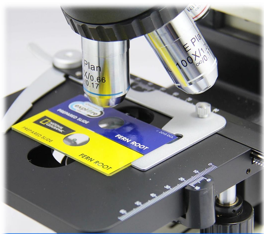
Mechanical Stage Size 145 × 140mm Travel Range 76 × 52mm
