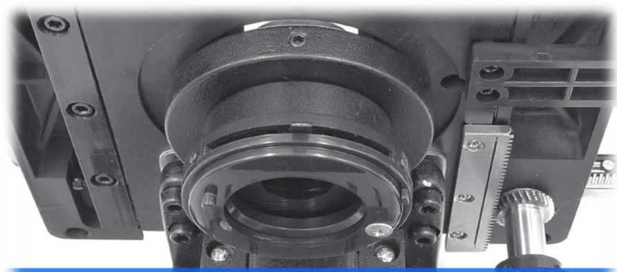
Abbe Condenser N.A.1.25, Iris Diaphragm, Rack & Pinion Up/Down
